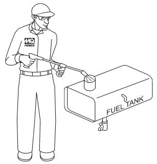
Figure 59. Fuel Tank Cleaning
